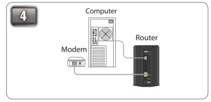
Unplug the Ethernet cable from your modem (or Plug one end of the included blue Ethernet cable that came with your router into the yellow port labeled INTERNET on the back of the router. Plug the other end of this cable into the Ethernet port on your modem.
